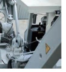
The hydraulically driven cable winch offers stepless and precise control of the load hook. Lowering the load occurs while stress flows constantly. If the cable winch is not being used, the automatic safety brake is applied immediately and thus guarantees secure holding of the load.
